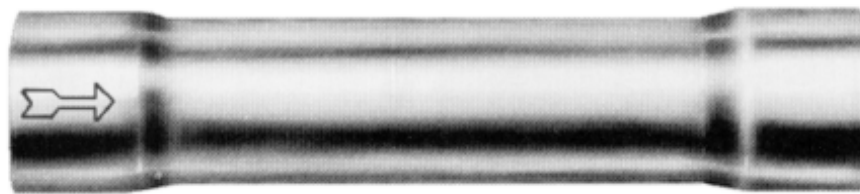
Dole Automatic Flow Regulator (actual size) 4 1 / 2 " long with 3 / 4 " sweat connection
